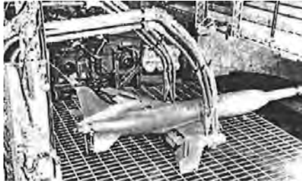
Figure 39.20 - Model with engines mounted under the wing - Lockheed 1011. Source: T.M.D. Sutton, Rolls-Royce. Aircraft Engineering, March 1976
