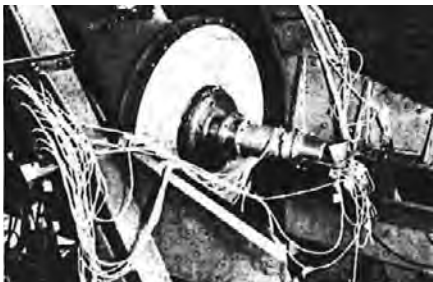
Figure 39.18 - Target type thrust reverser. Source: T.M.D. Sutton, Rolls Royce. Aircraft Engineering, March 1976
