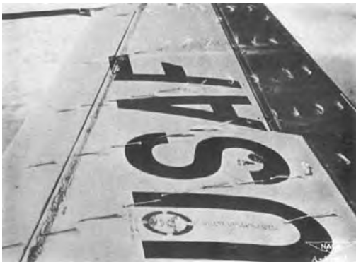
Figure 21.6 - Wing at M = 0.87 and C_{Na} = 0.49 . Source: NACA RM A52A31
