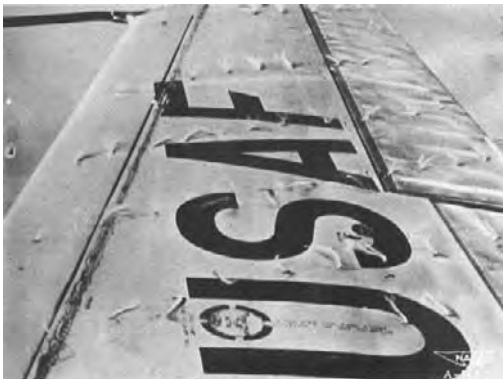
Figure 21.7 - Wing at M = 0.87 and C_{Na} = 0.74 . Source: NACA RM A52A31
