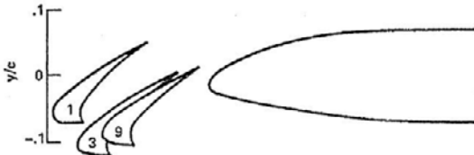
Figure 25.11 - Changing slat position to improve the pressure distribution on an airfoil section with a slat and a flap at \alpha = 15 \text{ deg} and \delta_i = 10 \text{ deg} . Re = 3.8 \times 10^6 . Source: NASA TM 78566
