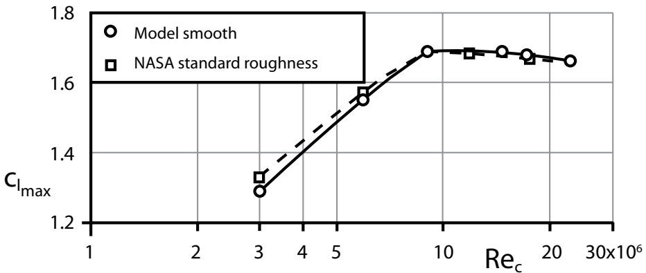
Figure 19.9 - Variation of maximum lift coefficient with Reynolds number at Mach 0.22. Source: NASA TMX-3160
