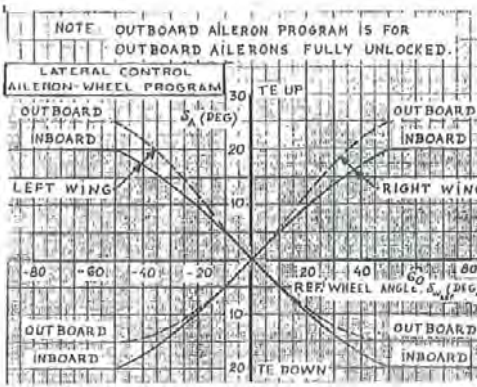
Figure 34.13 - Gearing between control wheel and roll control surfaces - Boeing 747-100. Source: NASA CR-114494
