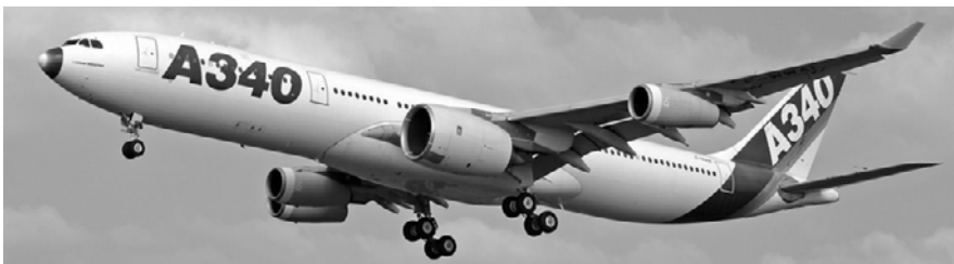
Figure 38.1 - Airbus A340 fitted with the engine of the A380. Source: Jorge Abreu
