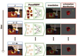
Left is Xinke Deng in the laboratory. The graphic shows an overview of the the PoseRBPF framework for 6D object pose tracking. The method leverages a Rao-Blackwellized particle filter and an auto-encoder network to estimate the 3D translation and a full distribution of the 3D rotation of a target object from a video sequence.
