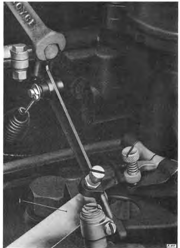
Fig. K14 Setting throttle lever -- S1 cars
