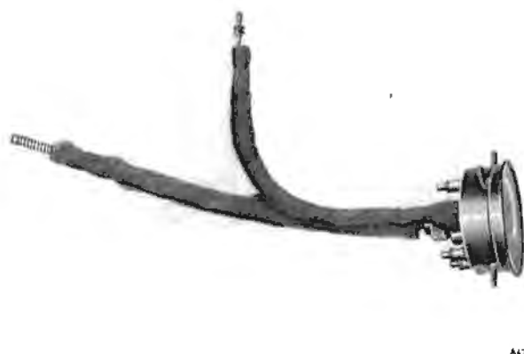
Fig. S44 Method of attaching anti-rattle felts to the speedometer cable and trip winder
