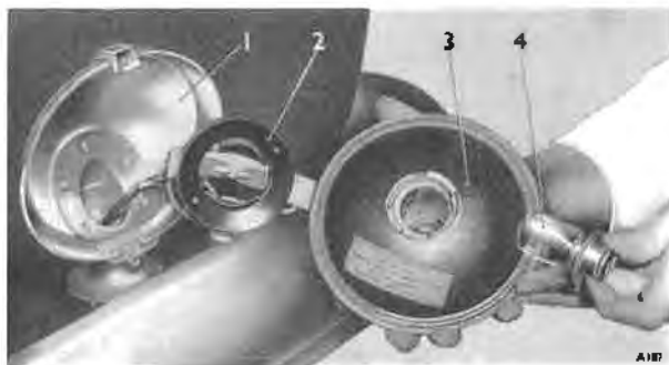
Fig. M45 Access to fog lamp bulb
