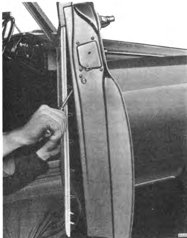
Fig. S1 Removing the trim from the front door
