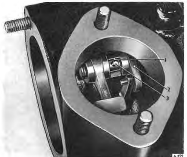
Fig. K18 Pick-up lever clearance — S1 cars
