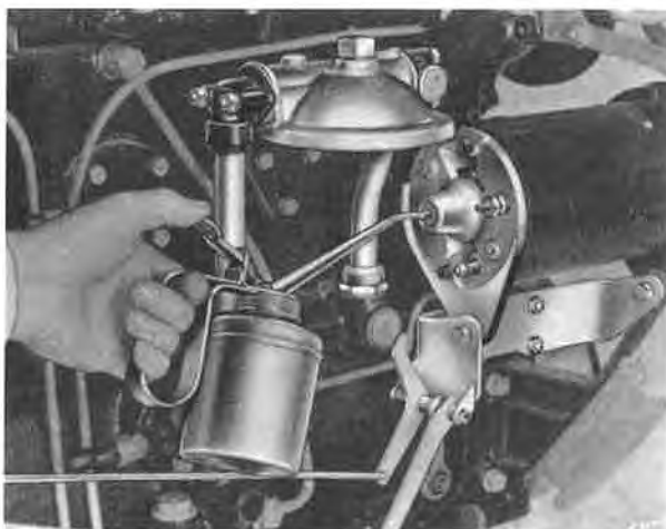
Fig. M4 Oiling commutator end bearing — C47 PV generator
