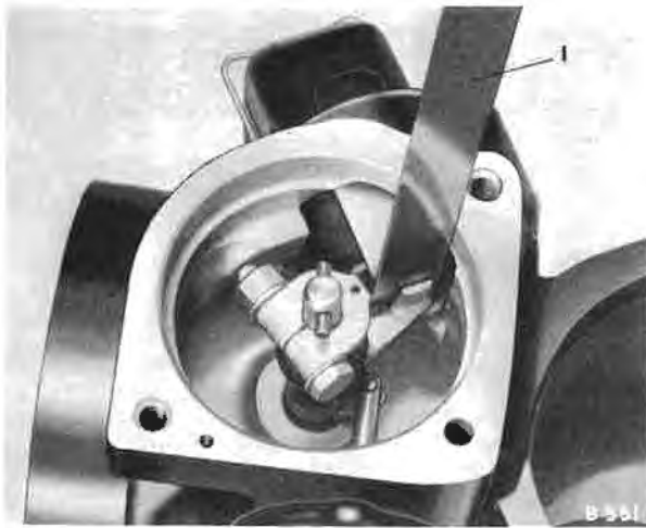
Fig. K21 Solenoid adjustment — S2 cars
