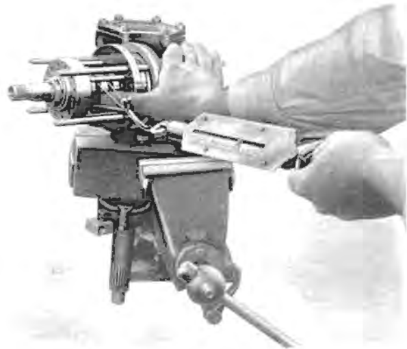
Fig. N28 Re-checking cross-load on spool valve
