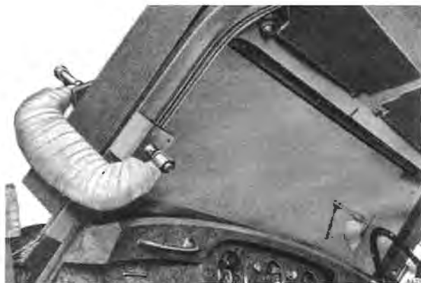
Fig. S50 Front seat showing the slide release and individual backrest rake
