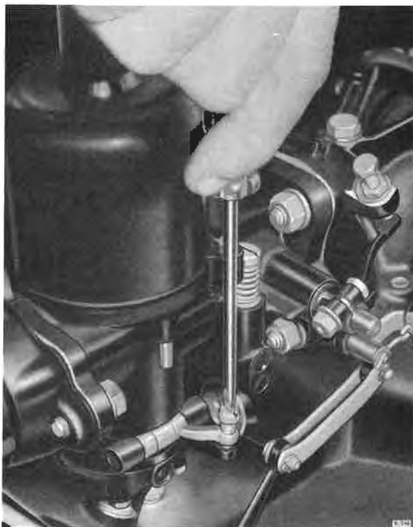
Fig. K25 Adjusting mixture control
