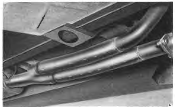
Fig. Q6 Position of exhaust pipe lagging
