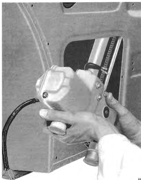
Fig. S17 Method of removing the mechanism assembly from the left-hand rear door
