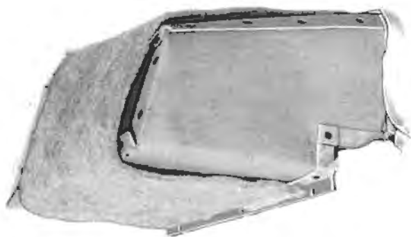
Fig. S41 Method of attaching anti-rattle felt to the cubby box
