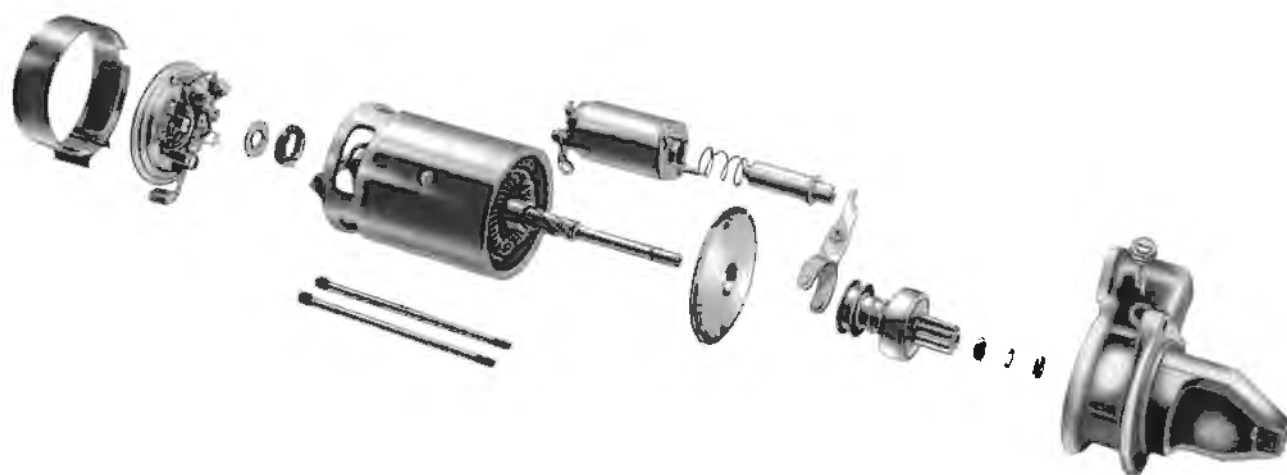
Fig. M26 Exploded view of starter motor — S2 cars
