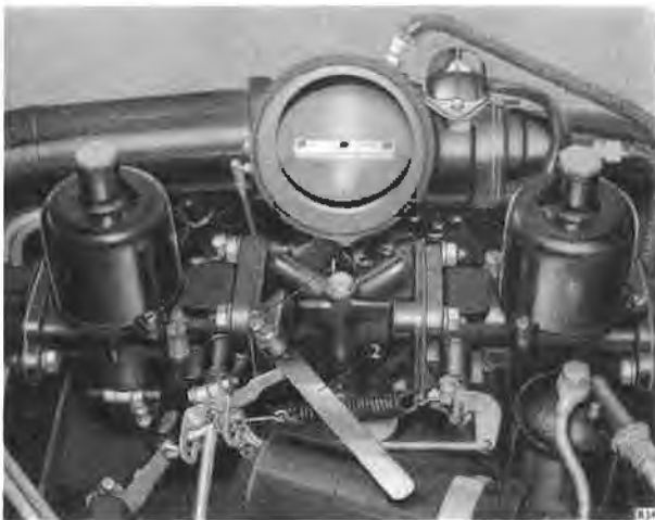
Fig. K15 Setting throttle lever — S2 cars
