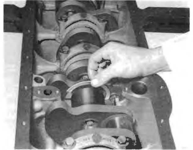
Fig. E15 Re-fitting thrust washers
