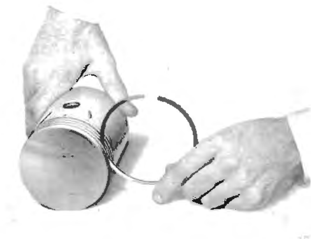
Fig. E22 Checking freedom of piston ring
