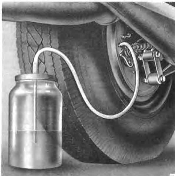
Fig. G4 'Bleeding' rear brakes
