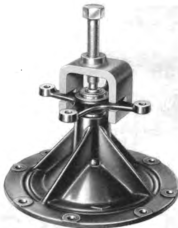
Fig. 1.18 Extractor - Coolant pump driving spider (S2 cars) (RH.7099)
