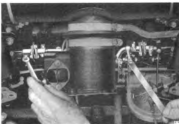
Fig. K13 Synchronising throttles — S1 cars
