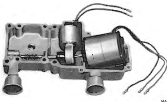
Fig. S22 Method of removing electric motor from the casing
