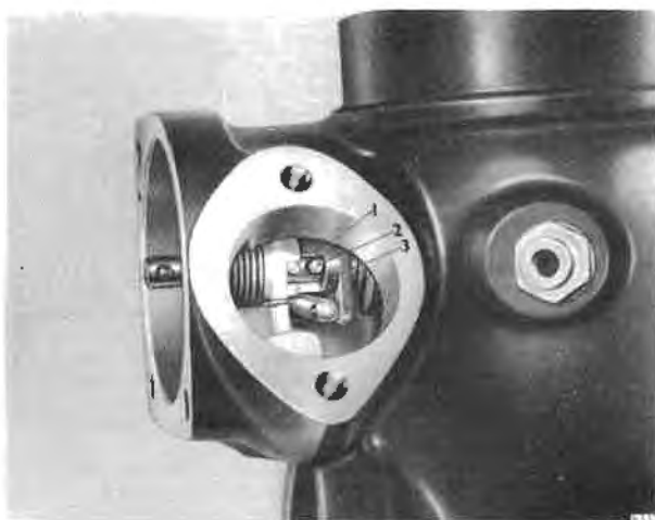
Fig. K19 Pick-up lever clearance — S2 cars
