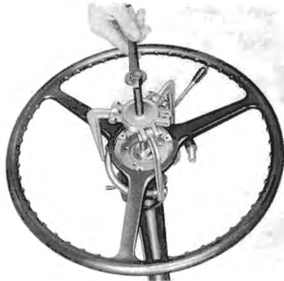
Fig. N18 Removing steering wheel
