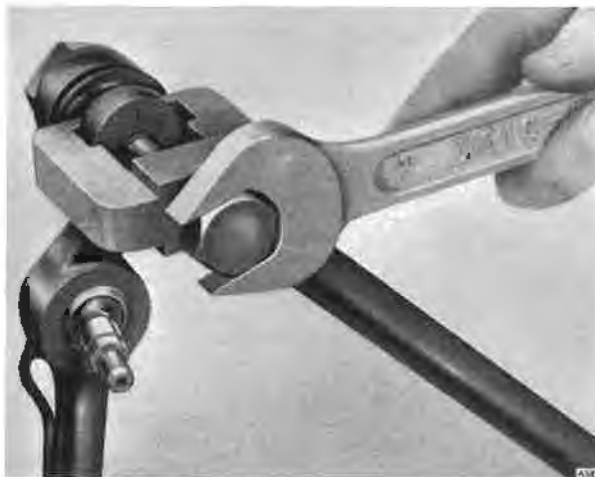
Fig. N12 Removing ball pin
