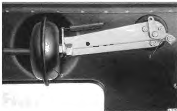
Fig. C9 Butterfly valve actuating mechanism
