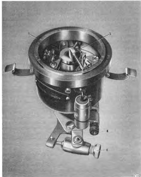
Fig. M35 Synchronising tool in position — S2 cars
