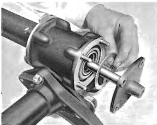
Fig. N21 Steering box lower adjusting washer
