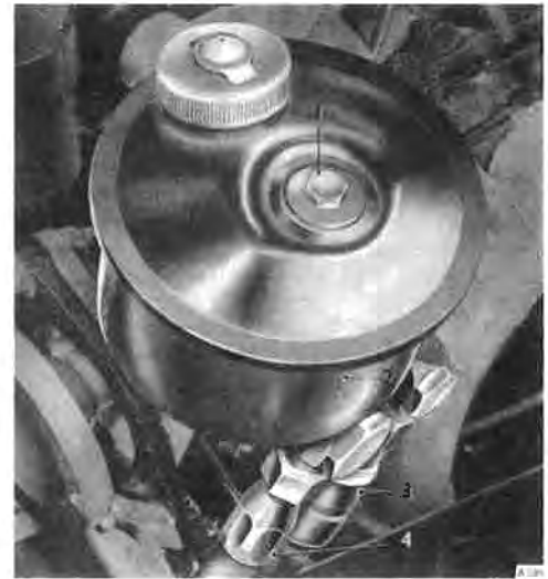
Fig. N7 Steering pump reservoir and filler cap
