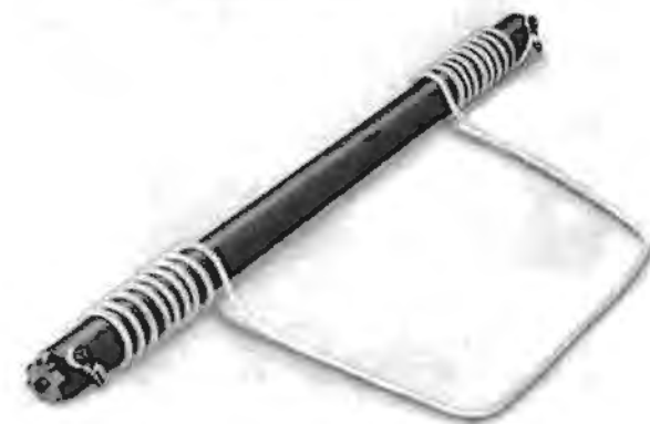
Fig. S34 Spring-loaded roller and nylon cord
