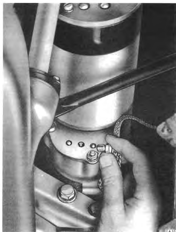
Fig. M21 Filling starter reduction gear casing — S1 cars
