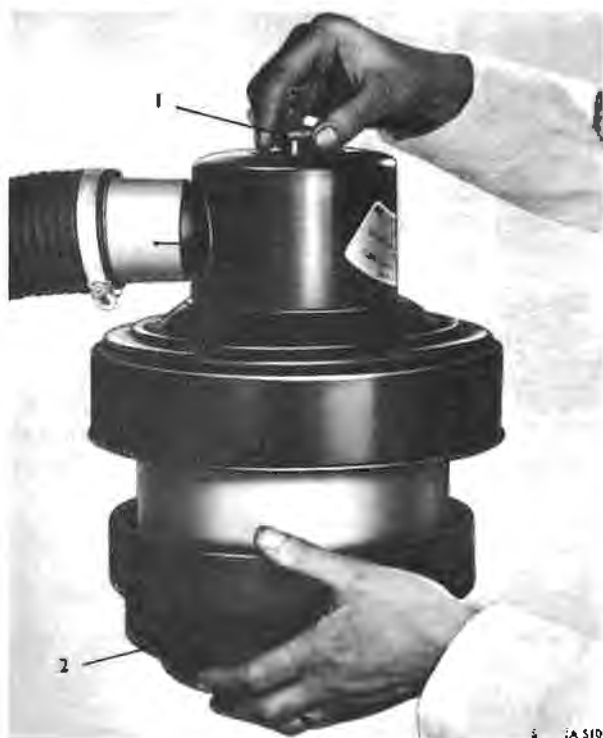
Fig. K8 Removing oil bath air cleaner — S1 cars
