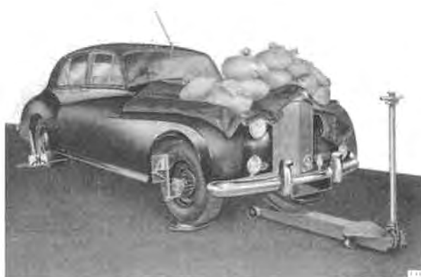
Fig. H10 Car loaded with jack in position
