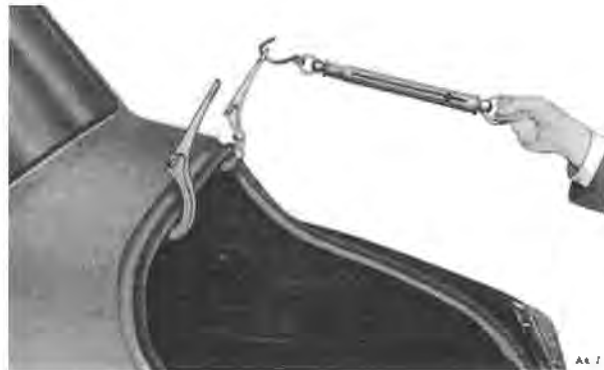
Fig. S36 Checking the luggage boot lid assistor poundage
