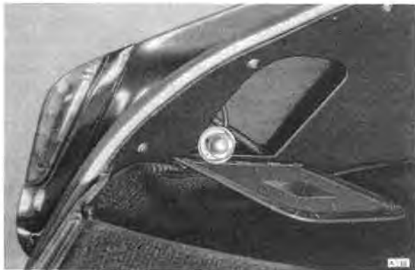
Fig. M46 Access to stop and tail lamp bulbs
