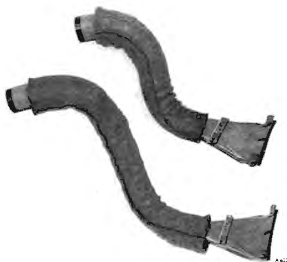
Fig. S43 Method of attaching anti-rattle felts to the de-mister ducts
