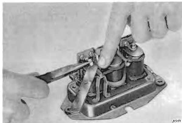
Fig. M17 Adjusting cut-out armature back stop
