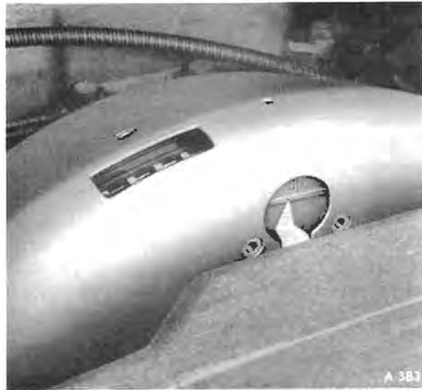
Fig. E8 Flywheel timing mark
