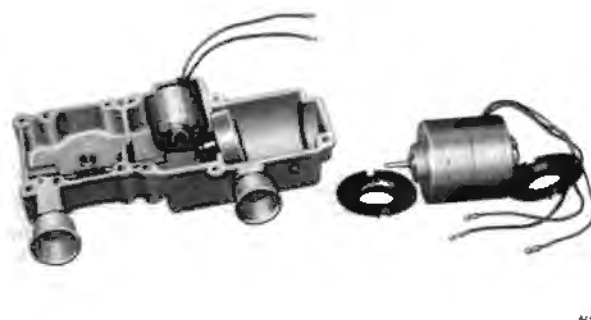
Fig. S23 Method of removing the flexible coupling from the casing
