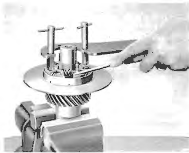
Fig. E20 Re-fitting drive springs
