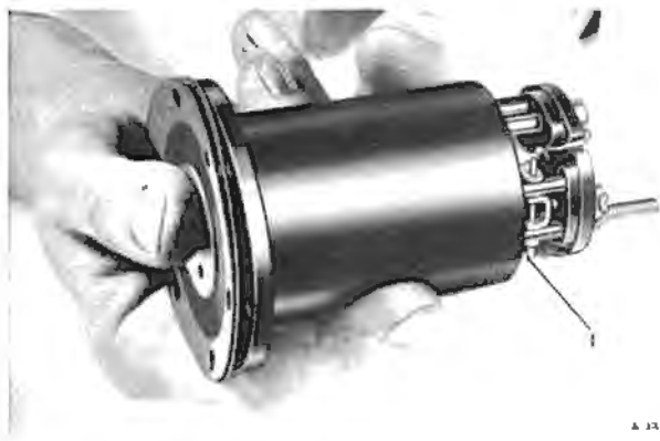
Fig. K6 Adjusting the diaphragm
