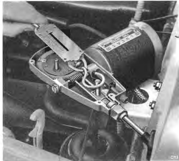
Fig. M50 Windscreen wiper load test
