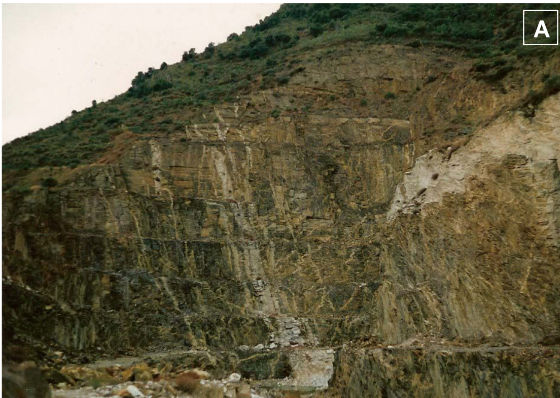
Stop 1: A) General view of the wall of the Feli open-pit (Fregeneda-Almendra) with a Li-mica rich subvertical dike, branched in its upper part, cross-cutting some cassiterite-bearing quartz-rich, folded veins.
