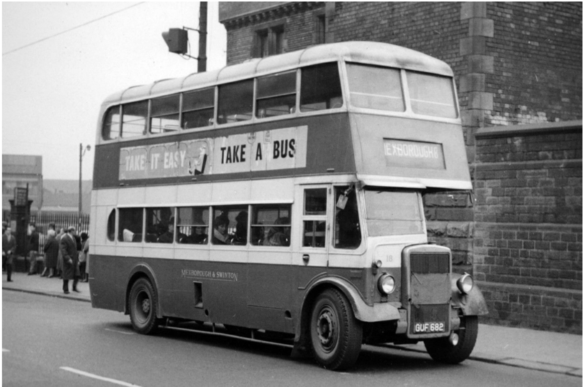
No. 18 (GUF682) was a 1946 Leyland PD1 with Park Royal 58-seat bodywork, new to Southdown Motor Services as No. 282, that joined the fleet in 1963. It was withdrawn in 1966. (LTHL collection).
