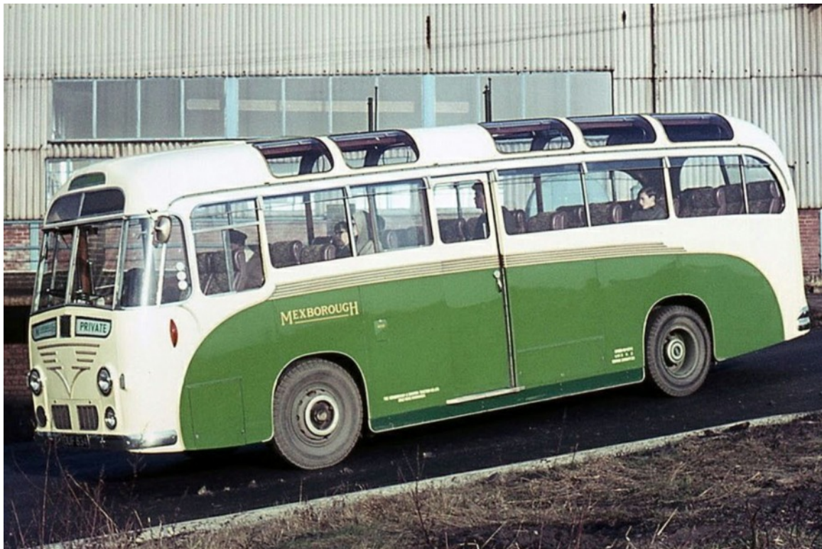
No. 103 (OUF834) was a 1955 Leyland PSUC1/16 with Harrington 26-seat bodywork that was formerly Southdown No. 1834. It was withdrawn in 1968. (LTHL collection).
