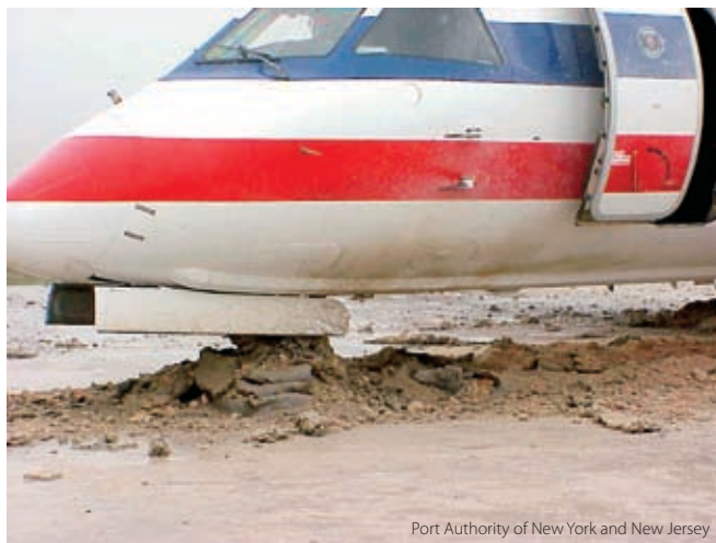
A Saab 340B arrestment occurred in 1999 at John F. Kennedy International Airport.
