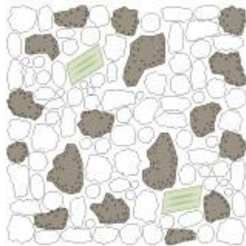
(c) Lithic sandstone: rock-fragment-rich
