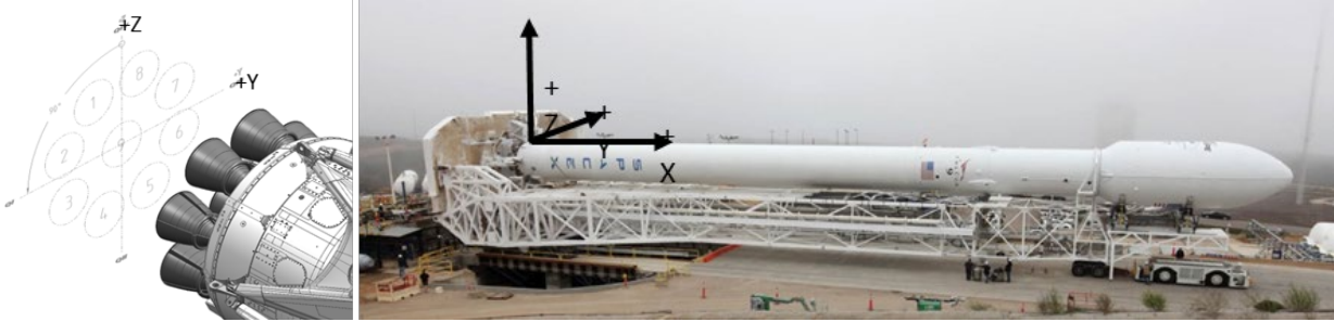
Figure 2-4: Falcon vehicle coordinate frame
