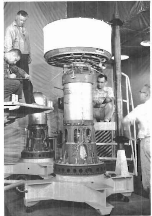
Tiros 1 was the first experimental meteorological satellite that introduced photography of earth's cloud cover from orbit.
