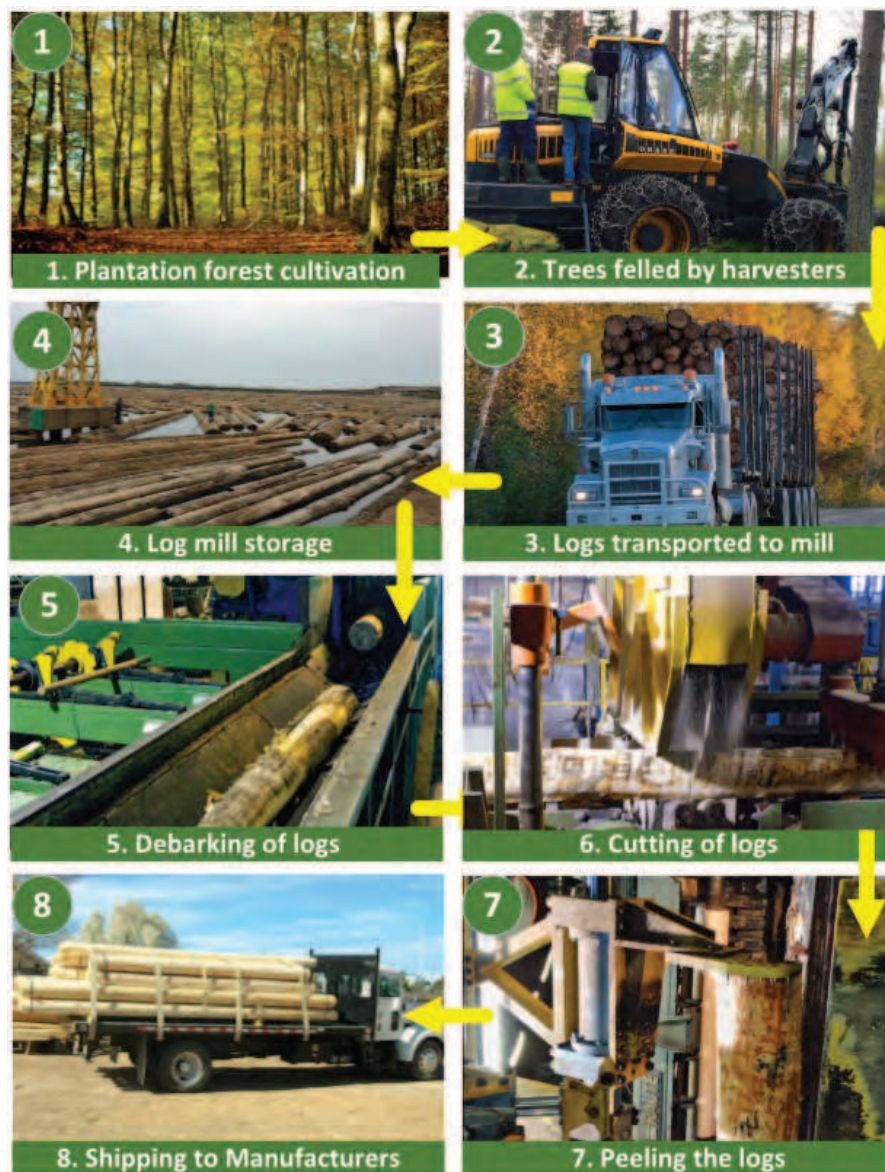
Figure 18.5. Steps in Modular (Knockdown) Furniture Manufacturing
