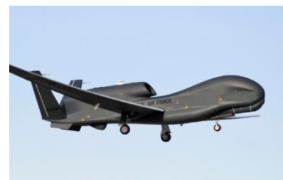
Long-endurance unmanned aerial vehicle (RQ-4B) Global Hawk (picture: same type of UAV)
