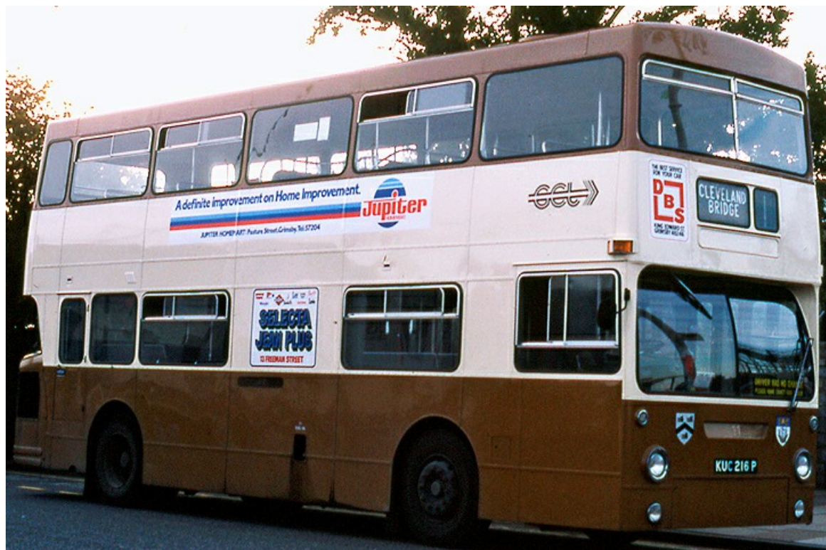
No.11 (KUC216P) was one of a number of Daimler CRL6's purchased from London Transport in 1981 and 1982. It carried a Park Royal 71-seat body and is seen here in September 1982 wearing the later caramel and cream livery. (LTHL collection).
