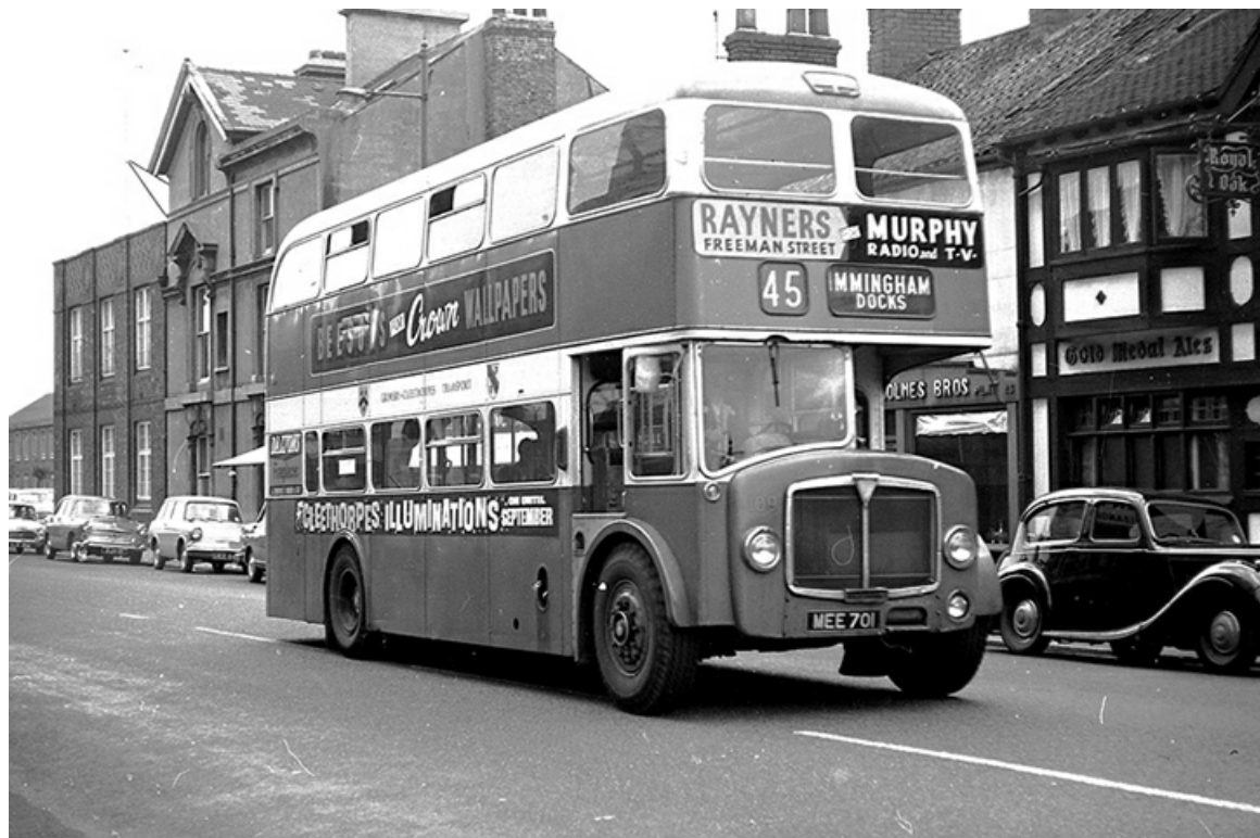
On its way to Immingham Docks is No. 109 (MEE701), a 1959 AEC Bridgemaster with Park Royal 68-seat bodywork. (Mike Beamish).
