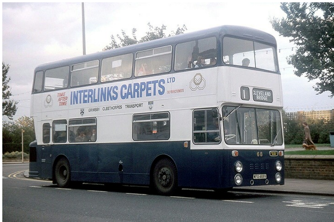
No. 68 (WFU468V), on its way to Cleveland Bridge, was a 1980 Leyland Fleetline with Roe 74-seat bodywork, wearing the darker blue livery. (LTHL collection).
