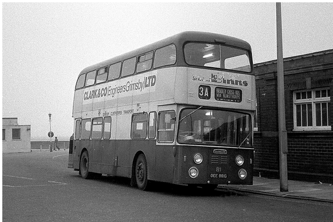
1969 Daimler CRG6LW No. 81 (OEE881G) with Roe 74-seat dual entrance/exit bodywork. (LTHL collection).
