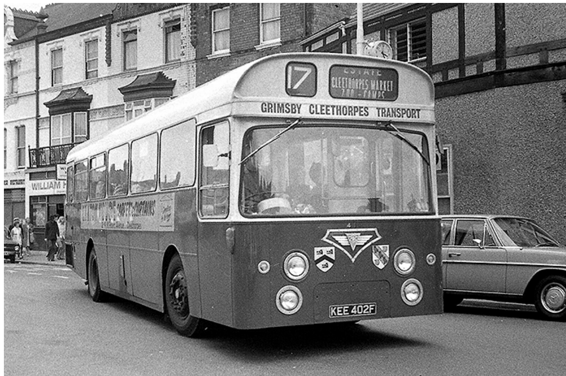
No. 41 (KEE402F) was a 1967 AEC Swift with Roe 42-seat bodywork, seen here heading for Cleethorpes. (LTHL collection).
