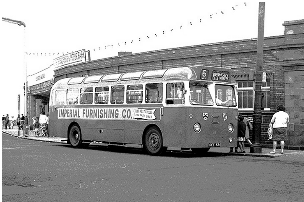
1961 AEC Reliance No. 18 (REE631) carried a Willowbrook 42-seat dual entrance/exit body. (LTHL collection).
