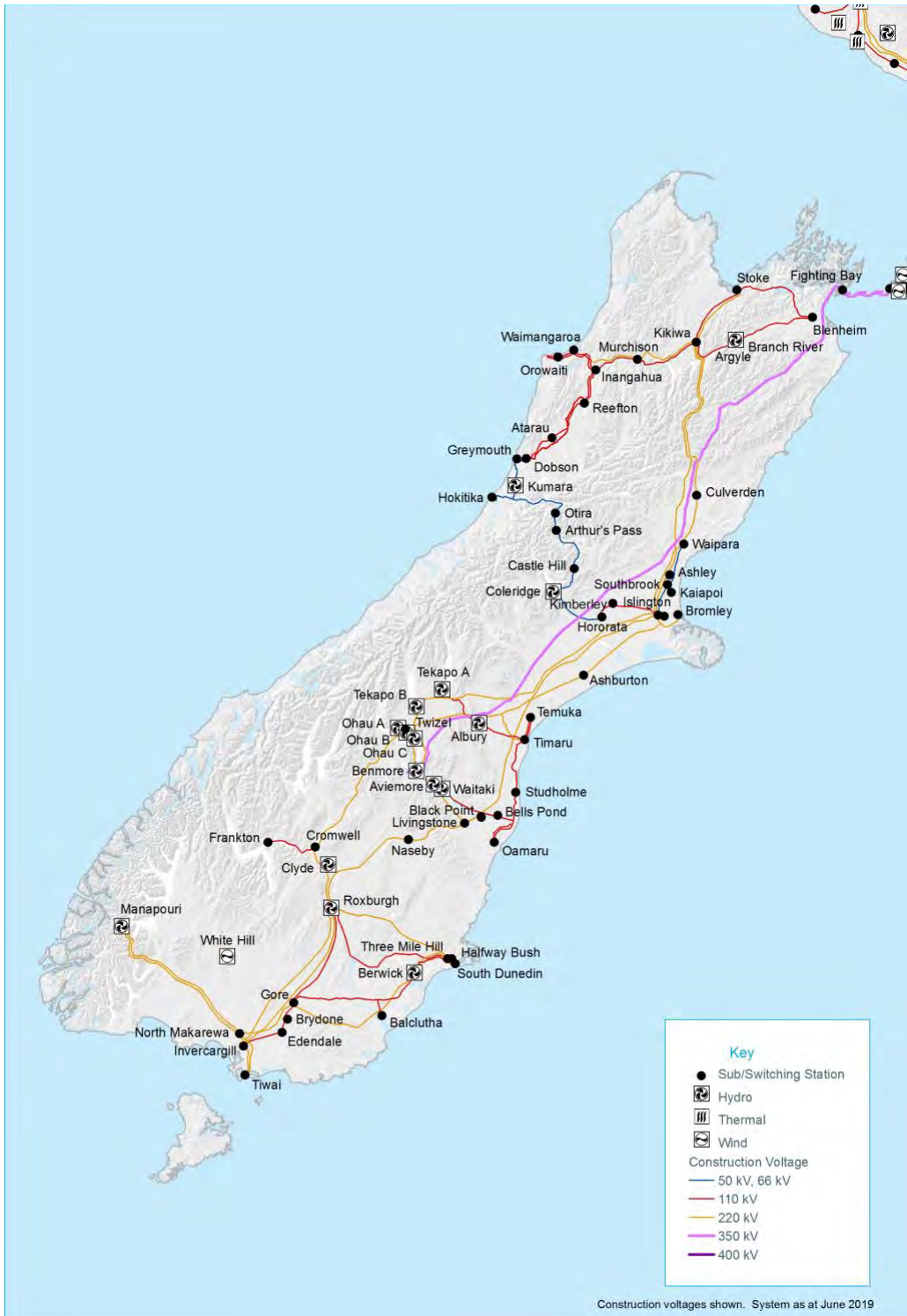
Figure 2-2: New Zealand's South Island transmission network
