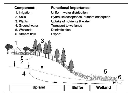
Schematic cross section of a land-based system for wastewater treatment employing upland and wetland components of landscape design
