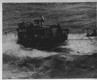
tomary way of Nazi scuttling. Another party from the Guadalcanal boards the foundering sub (above) and goes below to shut the scuttling valves. The men have to be shut up in the hull so seas won't pour down the hatch . . .
