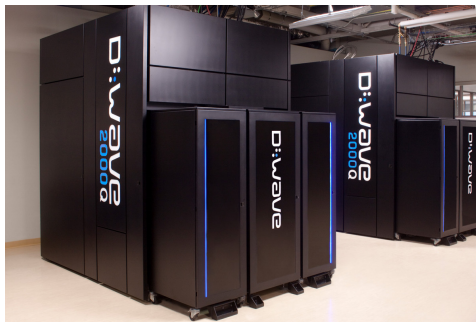
Figure 26.8: D-wave's room-sized 2000-qubit quantum annealing device.
