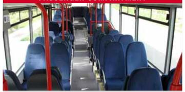
55 Fixed Brusa Divide seats including 4 tip-up seats and 1 movable double seat for increased access at centre door, fixed, steel armrests on aisle side and plastic anti vandalism seat backs
