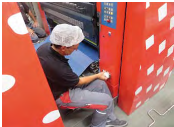
Blanket change on a Rapida 145: the blanket is registered by app on the printing unit on which it is used and its service life can be precisely tracked and planned.
