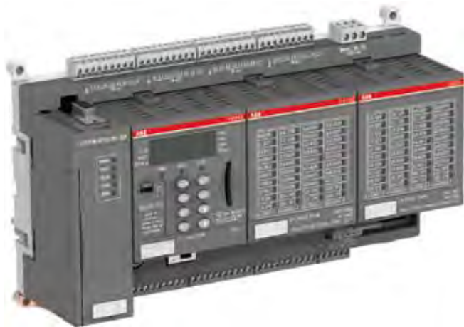
The ABB AC500 system mounted on the adapter that gives it footprint-compatibility with KT94 PLC.
