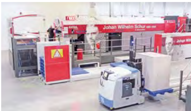
One of two Rapida 145s with double-pile delivery at Schur Pack Germany in Gallin.
