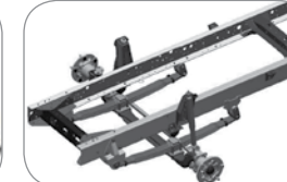
Front Parabolic Suspension and Rear Semi-elliptical Suspension
