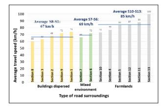
Figure 5 Travel speeds on sections with different types of surroundings
