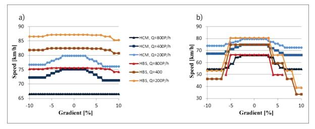
Figure 2 Impact of longitudinal gradient of road's on speed, with heavy vehicles share of traffic at: a) o %, b) 15 %
