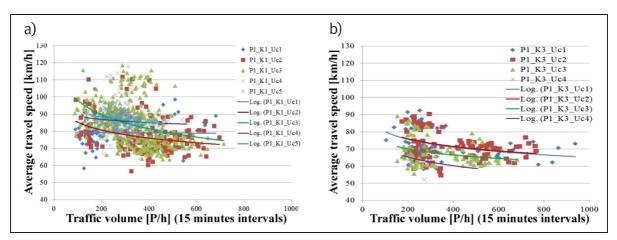
Figure 6 Travel speed depending on traffic volume in the primary direction and share of heavy vehicles for road curvature class/ vertical alignment class in HBS; a) 1/1, b) 3/1. Data from 38 research sites
