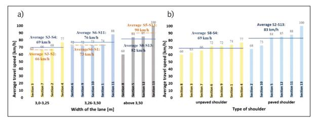
Figure 4 Travel speed on sections: a) of variable lane width, b) of variable type of shoulder
