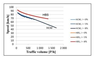
Figure 3 Impact of traffic volume on the analysed lane on vehicle speed
