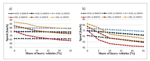
Figure 1 Impact of heavy vehicles on speed: a) flat terrain, b) longitudinal gradient 5 % (P/h – vehicles per hour)
