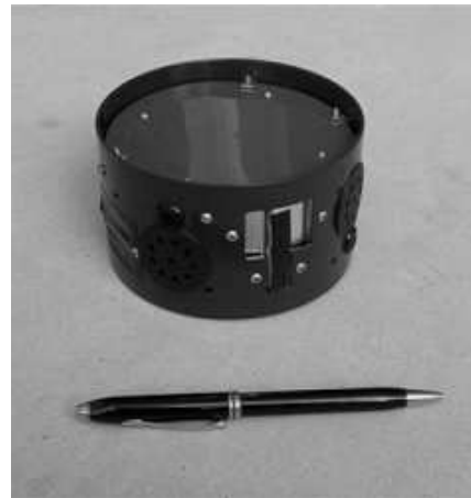
Figure 1: SHM node, which includes a stand-alone autonomous position location system shown next to a pen.
