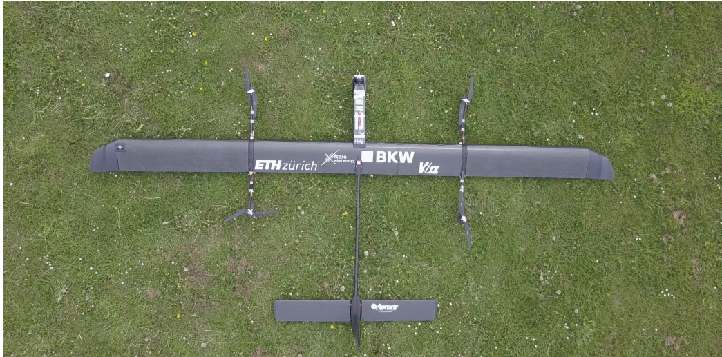
Figure 1: Prototype of focusproject fero with four propellers for VTOL
