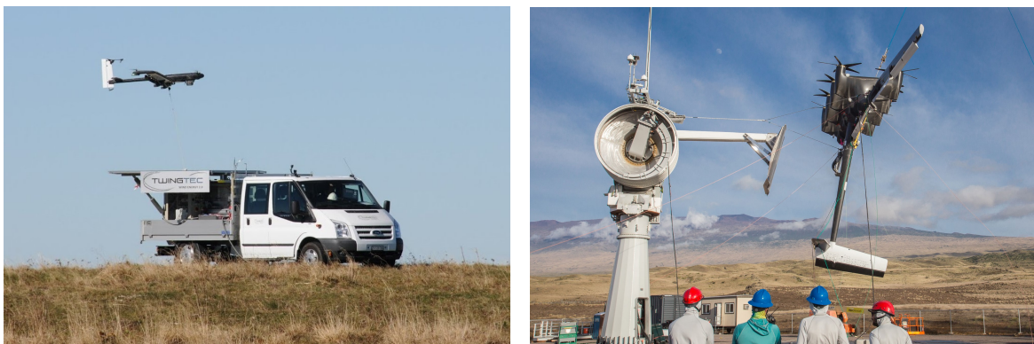
Figure 3: (a) Cross-wind AWE system employing VTOL from TwingTec [3], (b) on-board generating system using VTOL developed by Makani Power [4]
