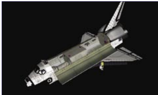
Figure 6.4-1. The speculative repair option would have sent astronauts hanging over the payload bay door to reach the left wing RCC panels using a ladder scavenged from the crew module.
