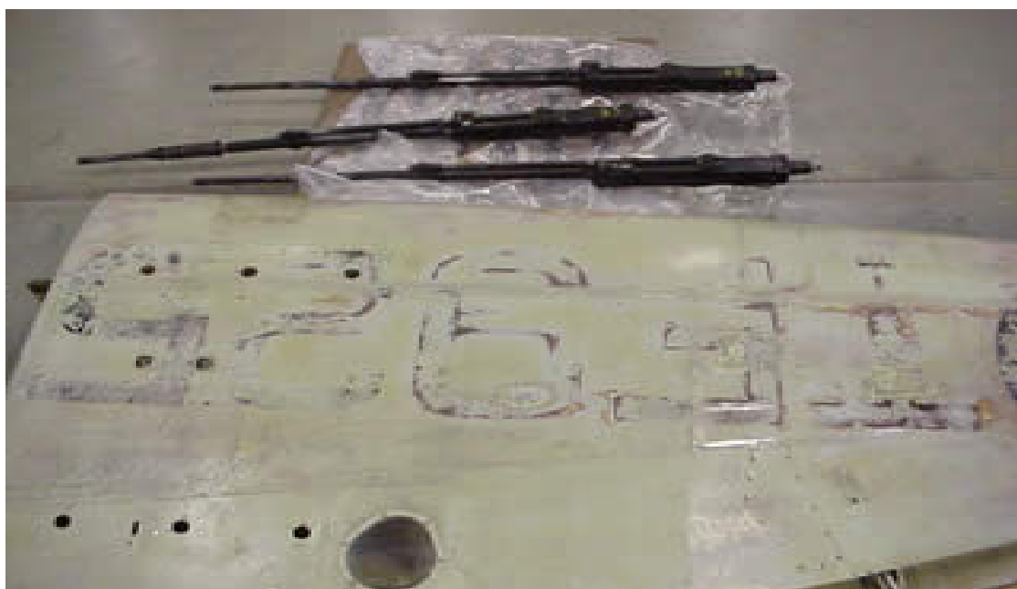
Figure 8. Port wing undersurface (note Hispano cannon).
