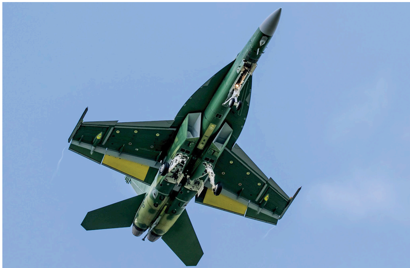
Captured on final of Lambert-St. Louis International (MO) after a testflight is F/A-18F 169751, the first Block III Super Hornet. This new version is capable of carrying shoulder-mounted conformal fuel tanks, among many other system improvements. (May 2020, Chase Kohler)
