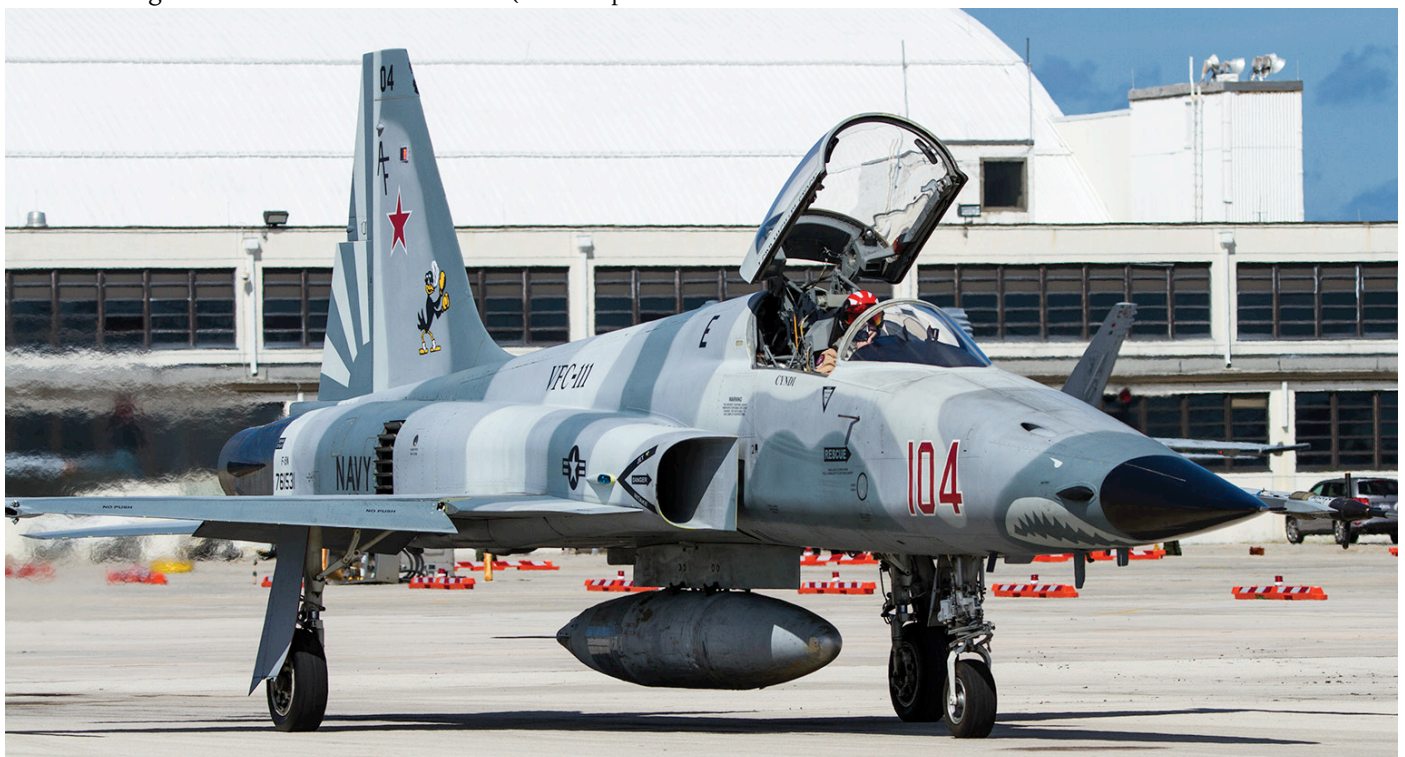
VFC-111 F-5N 761531 "AF-104" 2017 (3 tone gray scheme with lo-viz shark mouth and rudder markings). In order to be able to fly for a longer period of time, all the F-5s carry an external centreline fuel tank. The downside is that this tank degrades the performance of the aircraft in terms of G-forces. (George Karavantos)
