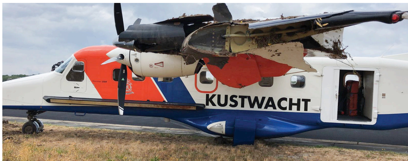
The Dutch Coast Guard Dornier 228 received what looks like minor damage after it suffered a burst left main gear tire at Eindhoven Air Base on 8 June. The runway at Eindhoven was closed for the rest of the day.
