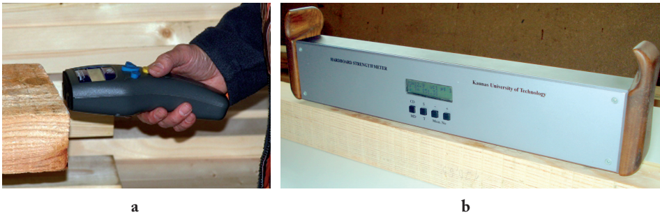
Fig. 1: Measurement devices: a – Timber Grader MTG (picture from http://www.brookhuis.com ): b – hardboard strength meter, developed at KTU
