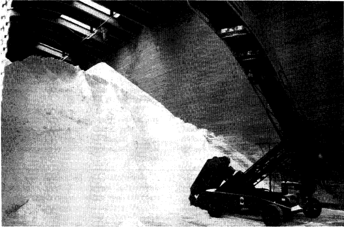
Figure 11. Conveyor Salt Loader in Switzerland.
