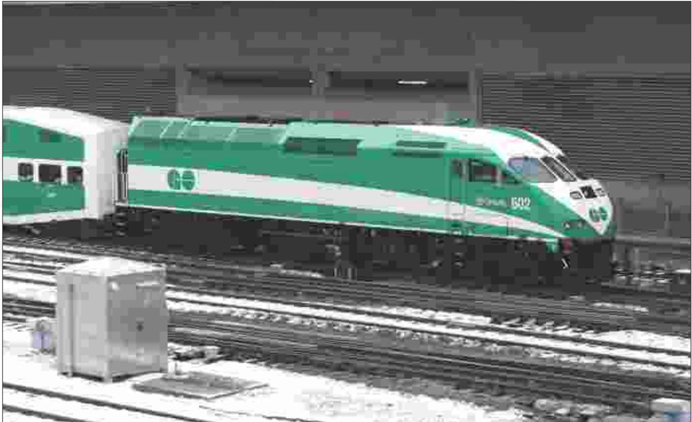
The new order arrives. MP40PH-3C 602 is westbound for the GO Transit servicing facility at Willowbrook near Mimico on January 15, 2008. Engine 602 is one of 27 new 4000 horsepower locomotives built for GO by Motive Power Industries of Boise, Idaho. Derek Boles.
