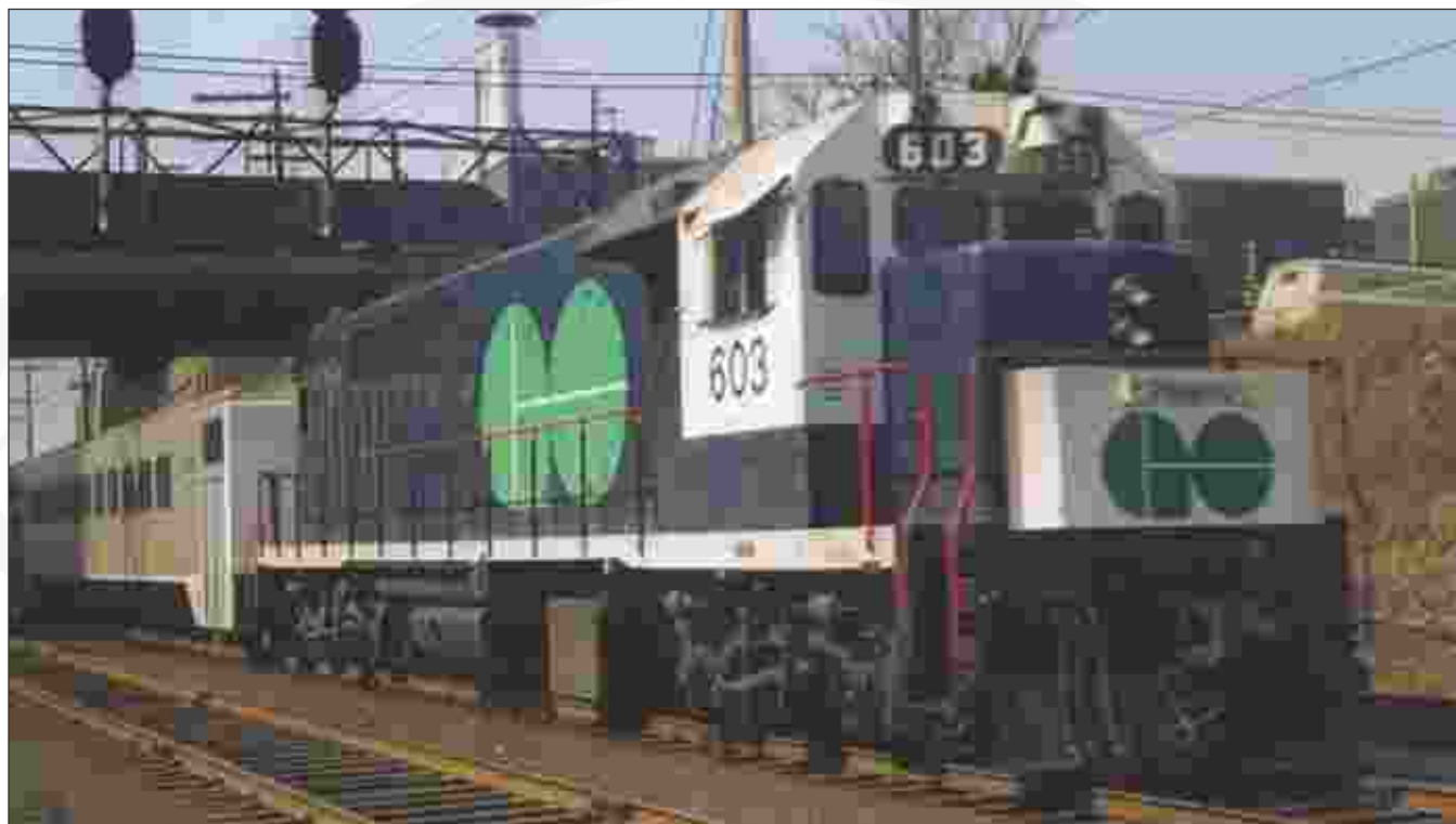
The first diesel-electric locomotives that powered GO Trains were 3000 horsepower GP-40TC's built by General Motors of London, Ontario. The ``TC`` in the GP-40TC model designation stood for ``Toronto Commuter``. In April 1969, GP-40TC 603 is eastbound for Pickering at Strachan Avenue in Toronto. Jurus Zvidris.
