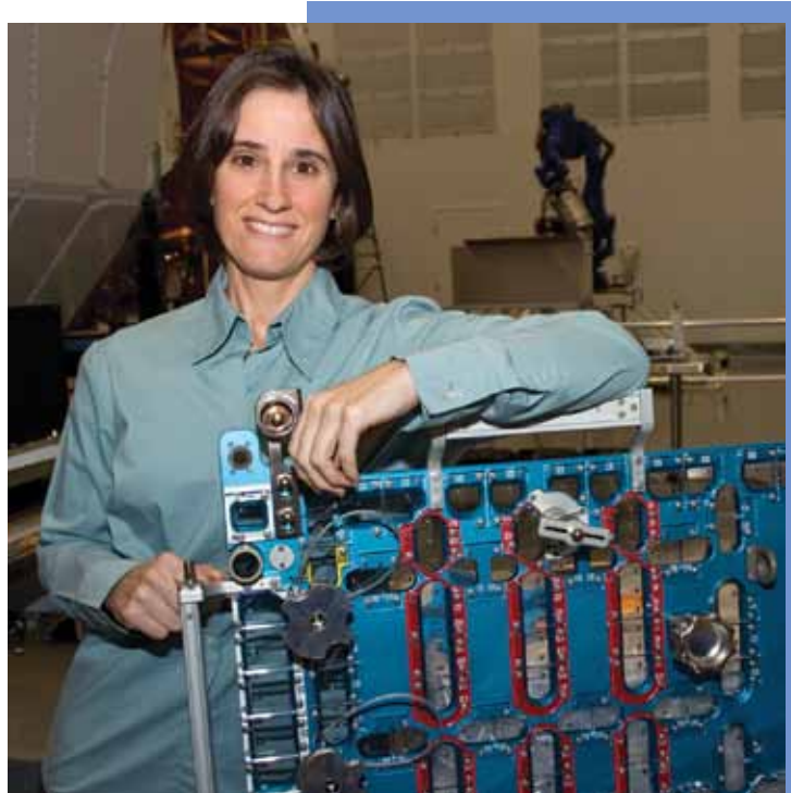
Lisa holding the Space Telescope Imaging Spectrograph (STIS) capture plate that the astronauts used during Servicing Mission 4 to remove the 111 screws of the instrument's Main Electronics Board cover plate, September 2010.
