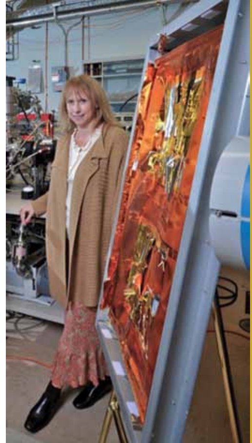
Nancy with returned Long Duration Exposure Facility (LDEF) hardware showing space environments materials damage, January 2011.
