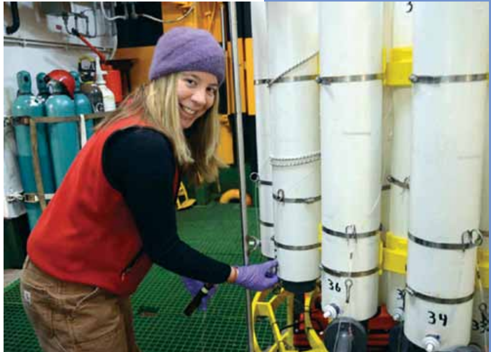
Aimee taking a seawater sample from the Conductivity-Temperature-Depth (CTD) rosette on the ship Nathaniel B. Palmer in the Southern Ocean, March 2011.
