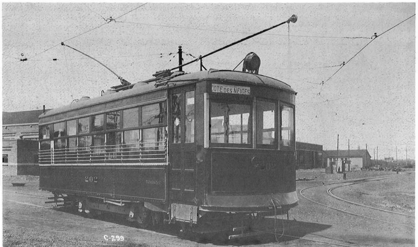
Before and after the Birneys came: The larger companies also benefited from the use of Birneys on outlying lines, as we can see in these two views on the Montreal Tramways system. The top view, taken in 1912, shows car 640, one of Montreal's earliest double-truck cars, originally built in 1900, as it looked after conversion to a double-ender for use on low density lines. The bottom photo was taken at Youville shops in 1924 and shows Birney 202, newly arrived from Detroit. The Birneys would soon replace old wooden cars like 640 on routes such as Cote des Neiges, which was then a short stub-end line.
