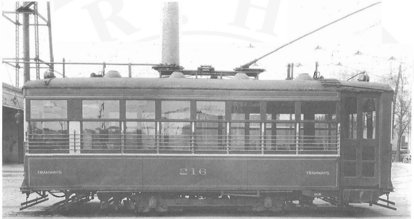
A broadside view of Montreal Birney car 216, photographed in 1931. This car had formerly been Detroit car 201, built in 1921, and it was scrapped in 1939.
