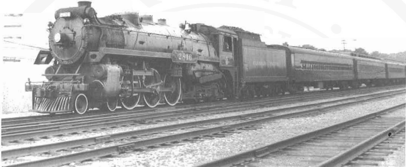
One of the last steam locomotives in Canadian commuter service was 2816, seen here between Westmount and Montreal West about 1960. Note that the first car is an 800 class. 2816, now known as the "Empress" is still in special excursion service on CPR lines in Canada and the United States. Collection of Peter Murphy
