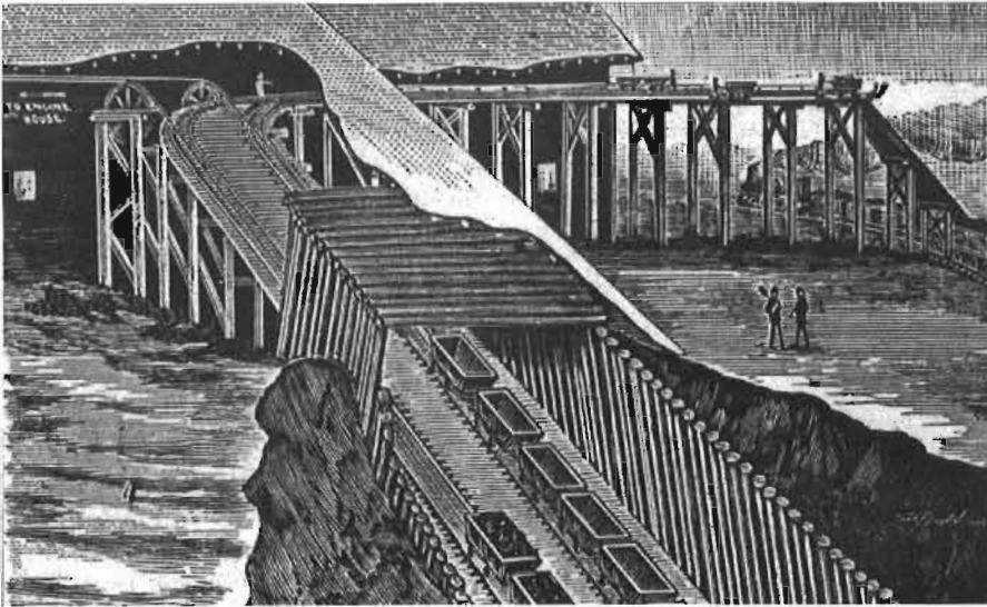
Illustration of a typical coal mine operation. The trains are loaded at the right. Taken from Morrow's history of the 1891 Springhill disaster.
