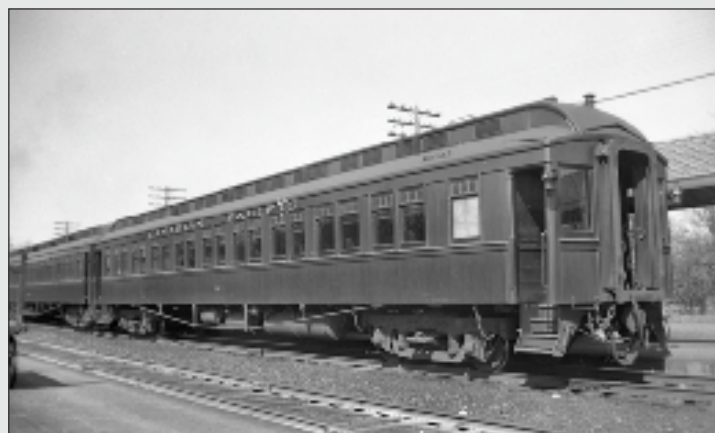
Canadian Pacific Railway's second generation commuter coach were still of wooden construction, but with closed vestibules. Coach 187 was in train # 573 operating between Montreal and Vaudreuil when this photo was taken on May 23, 1947. Ernest L. Modler, R. S. Ritchie Collection.
