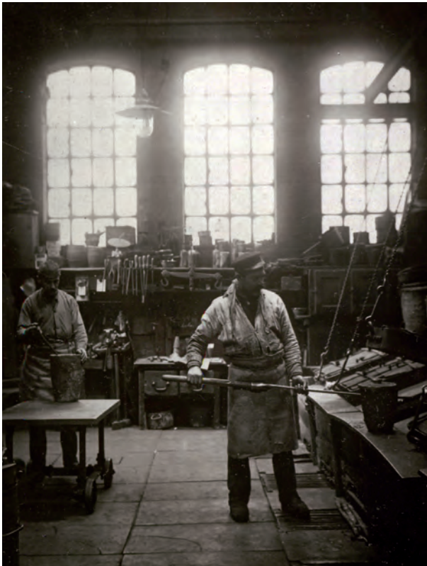
Workshop with coke-fired crucible furnace for melting precious metals at the Elbstrasse plant.
