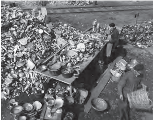
The metal objects donated by the population needed to be sorted. Scrap metal was piled several meters high on the NA works premises. Not only here but also at other smelting plants it was melted and supplied to the armaments industry.
