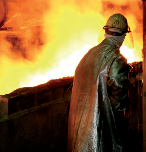
Metal tapping at the Kayser Recycling System (KRS) in Lünen. The plant melts mixed materials containing copper and precious metals coming from used electronic and computer end products. During tapping, the plug of the furnace is opened so the liquid metal, whose temperature exceeds 1,000 °C, can run out.
