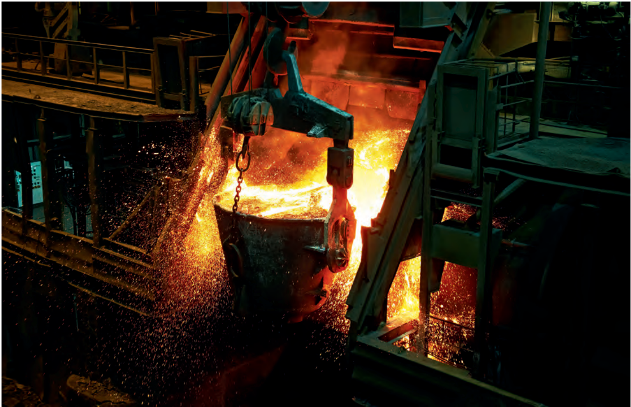
Charging of the converter with copper matte.
