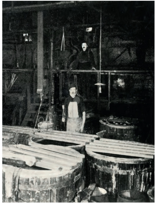
Wet chemical workshops at the vitriol smelter at Elbstrasse. This was the location where copper vitriol was produced. The foreground of the photo shows crystallization tanks hung with lead bars. Evaporating pans are standing on the platform in the background.
