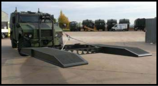
2: Light Support Bridge
