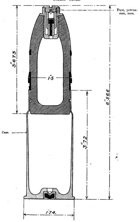
CARTRIDGE, Q.F., 1-PR., MARK I. STEEL SHELL.
