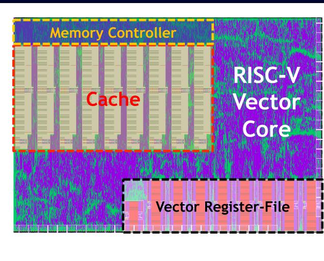
Fabricated in IBM 45nm SOI Runs at > 1GHz
