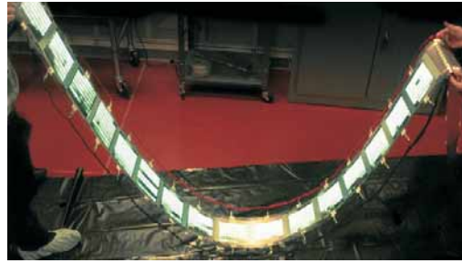
(b) A soft OLED lighting panel by GE from the US. (Source: [21])
