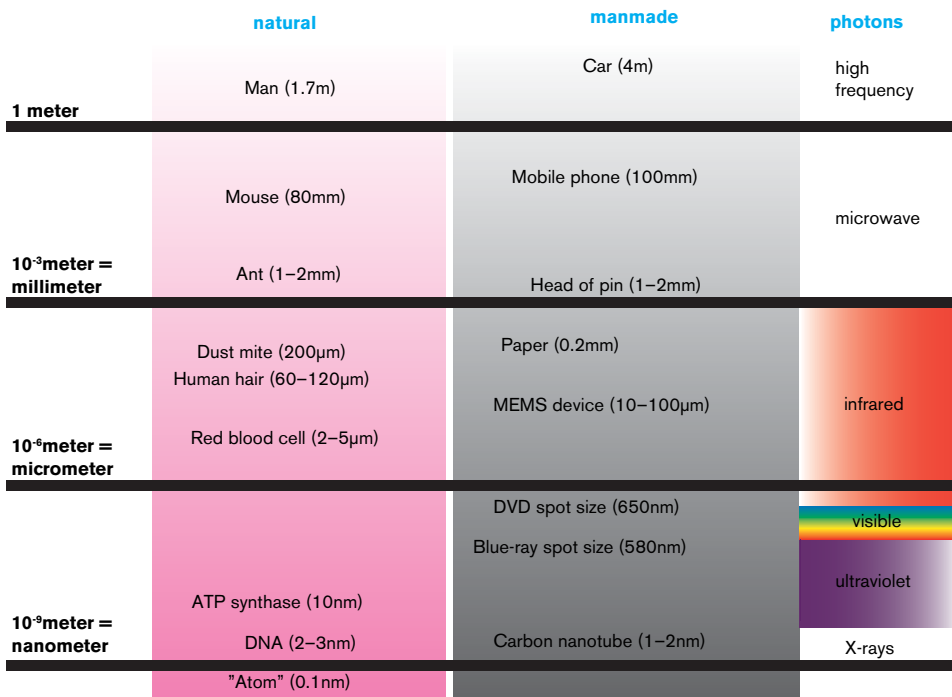
Figure 1. A comparison between natural and man made structures. Examples of nano level (at least one dimension less than 100 nm in diameter) structures are ATP synthase, DNA and Atom in natural category, and carbon nanotubes in man-made category.
