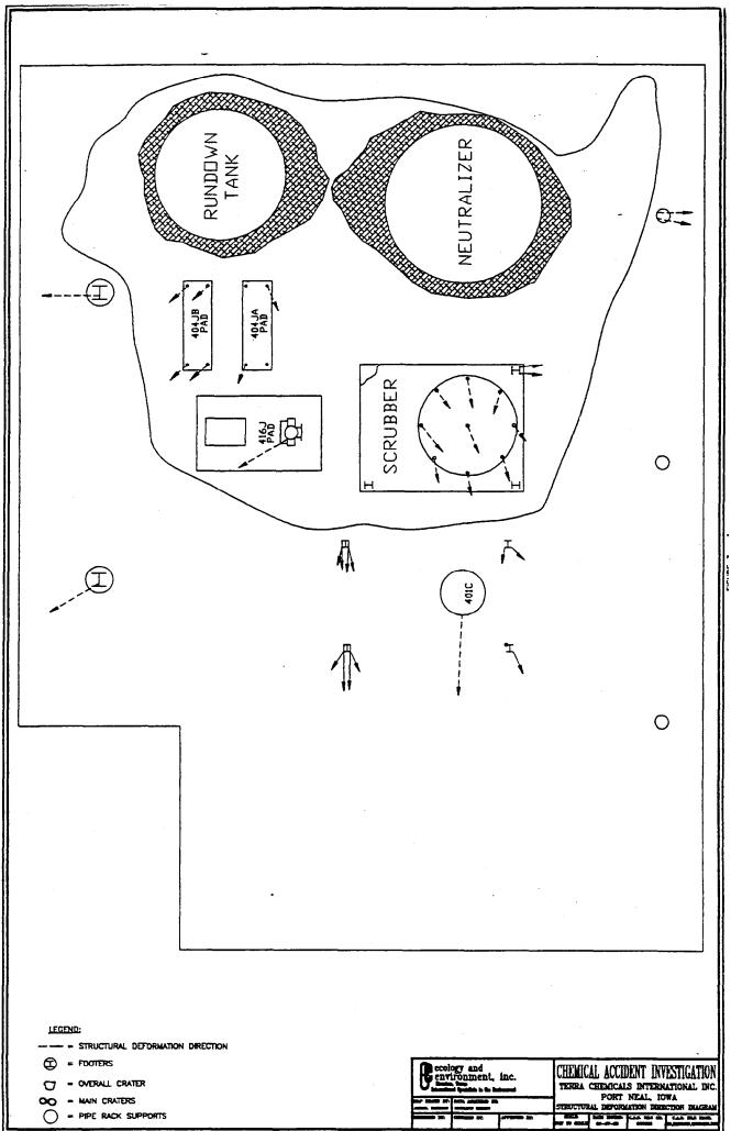
STRUCTURAL DEFORMATION DIRECTION DIAGRAM
