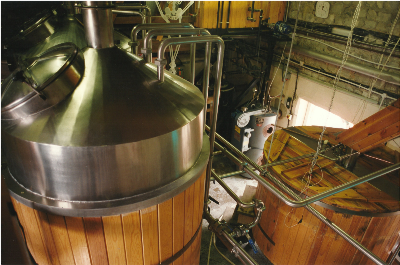
A modern micro-brewery: coppers and mash tun at the Hog's Back Brewery, Tongham.
