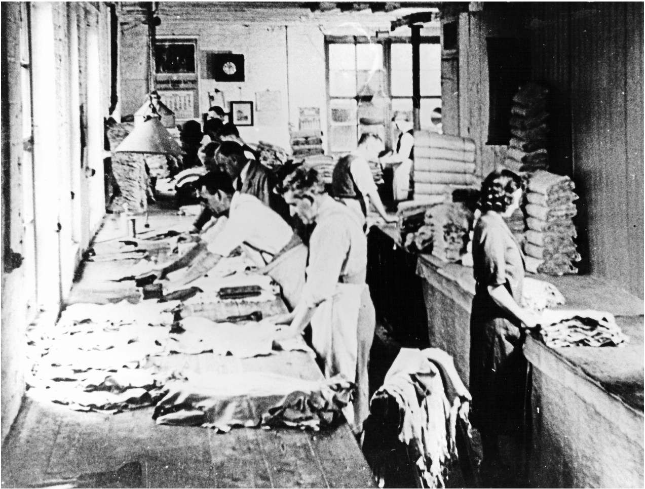
Workers stretching skins at Chuters' chamois leather works, Mitcham. Wandle Industrial Museum .
