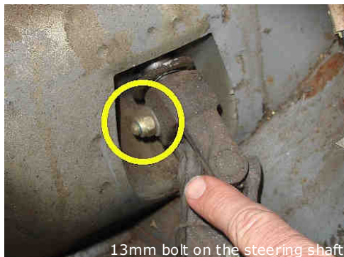
13mm bolt on the steering shaft
