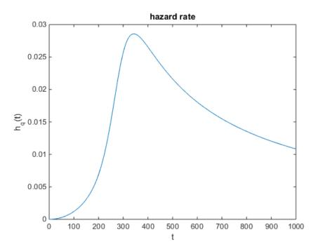
Figure 5-5: Hazard rate function for the two-motor system.
