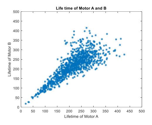
Figure 5-8: Simulated lifetime pairs of motor A and B.
