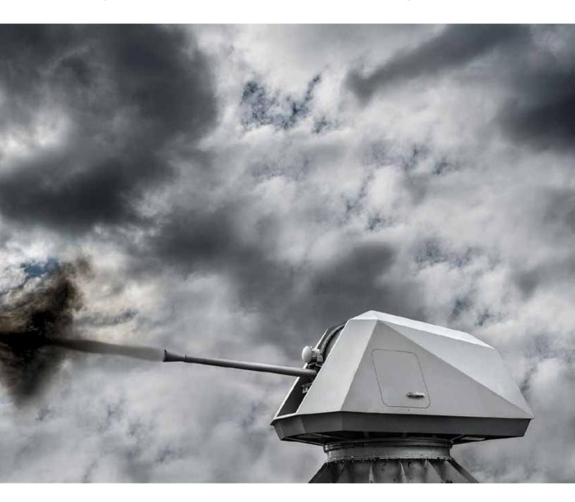
The Bofors 57 Mk3 naval gun system fires four rounds per second and can switch immediately between ammo types, including smart 3P all-target ammunition. This delivers seamless targeting of air, land and sea-based threats.
