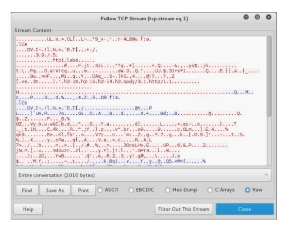
Figure 7-2: Follow TCP stream on SSL/TLS traffic
