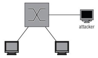
Figure 4-11: Capturing packets with a hub
