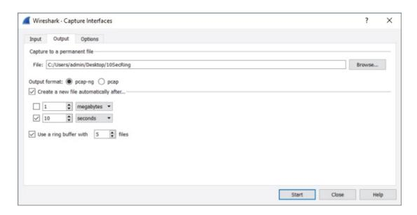
Figure 4-21: Setting multiple files and ring buffer
