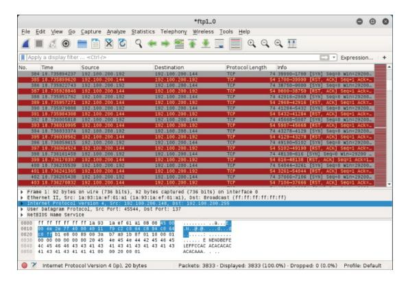
Figure 6-3: Nmap port scan in Wireshark
