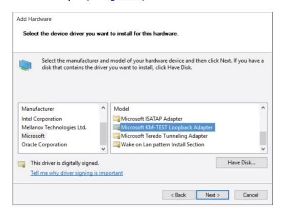
Figure 4-6: Installing the loopback adapter on Windows
