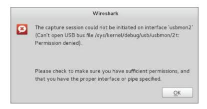
Figure 7-11: Wireshark usbmon error
