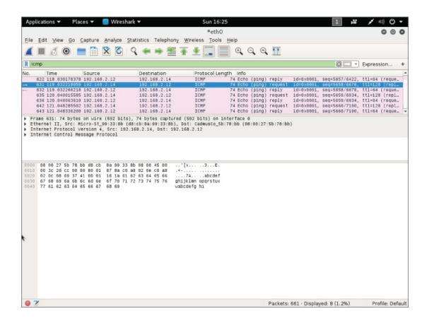
Figure 4-10: Wireshark sniffing bridged network
