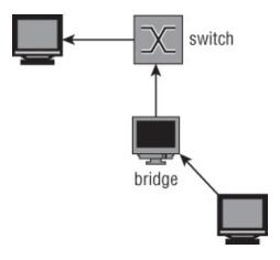
Figure 4-15: Traffic flow when sniffing a Linux bridge
