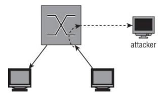
Figure 4-13: SPAN sniffing connections
