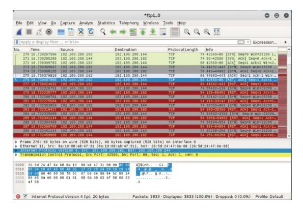
Figure 6-4: Open port in Wireshark
