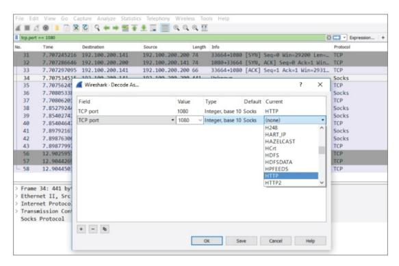
Figure 4-27: Wireshark's Decode As window
