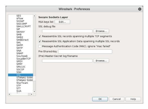
Figure 7-3: Wireshark SSL/TLS protocol options
