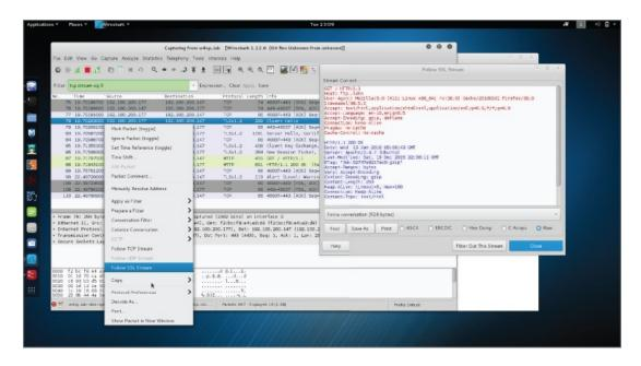
Figure 7-5: Decrypting TLS traffic in Wireshark
