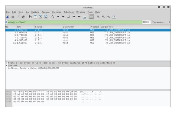
Figure 7-15: Filtering USB traffic to host
