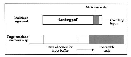
Figure 6.5: – stack smashing attack
