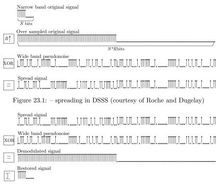
Figure 23.2: - unspreading in DSSS (courtesy of Roche and Dugelay)
