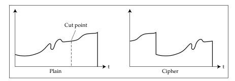
Figure 24.1: – cut-and-rotate scrambling
