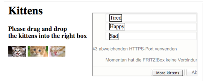
Fig. 1. UI redressing attack using the drag-and-drop API.
