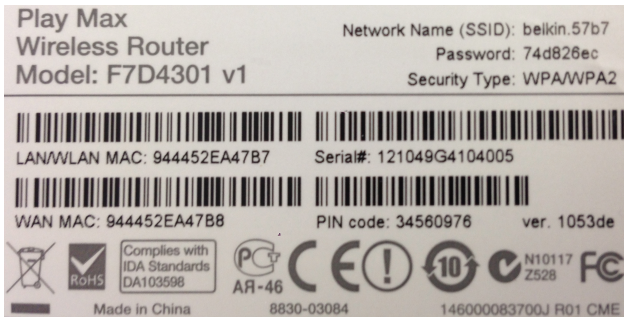
Fig. 2. A part of the label of the Belkin F7D4301 on the bottom of the device. On the top right one can see a probable randomly generated password.
