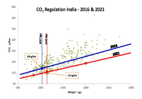
This regulation will be mandated for M1 category of motor vehicles (commonly known as the passenger vehicles, weighing below 3,500 kgs). Several measures would be taken by the industry to adopt the stringent fuel efficiency regulations such as improvement in engine efficiency, improvement in transmission efficiency, reduction of weight, use of alternative fuel, etc.
