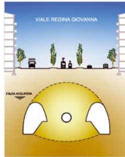
2 - Excavation of two side drifts for the sidewalls of the station tunnel
