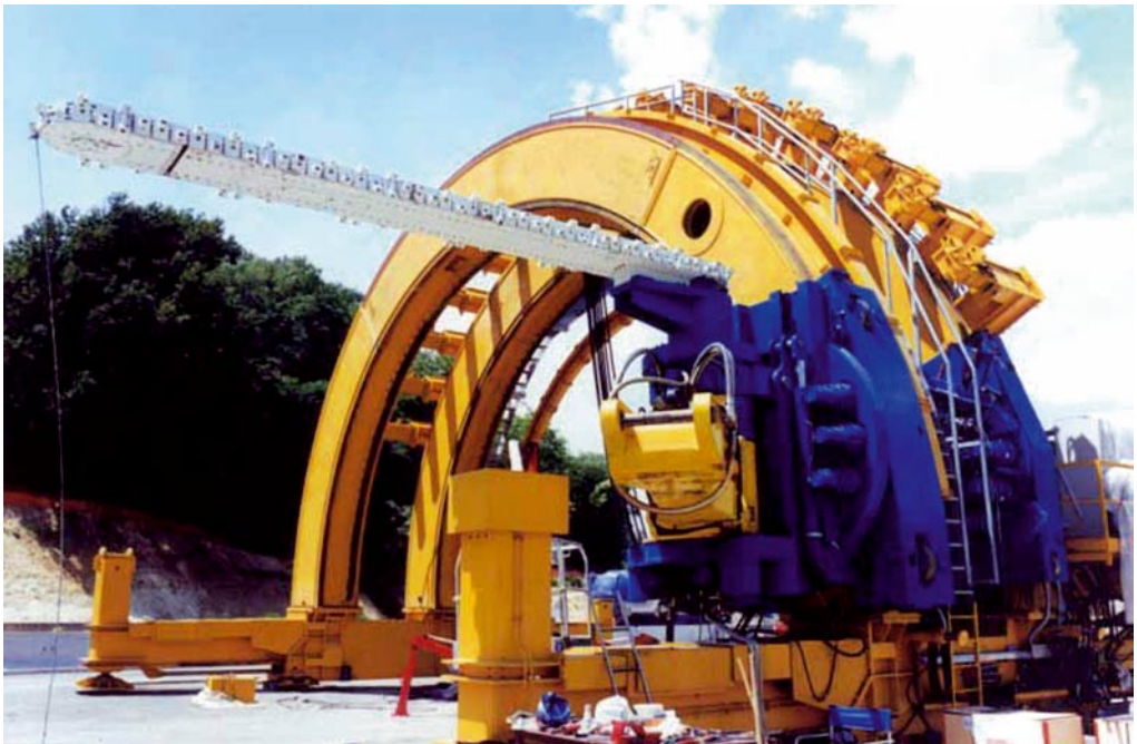
Fig. G.12 View of the machine with the large chain saw for making the precut in the foreground
