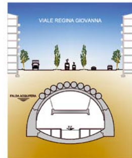
6 - The tunnel invert is cast and the mezzanine floors built with finishing works
