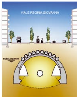
4 - The transverse arches are built working from inside the minitunnels
