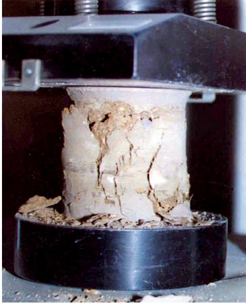
Fig. E.3 Test piece subjected to mono-axial compression test
