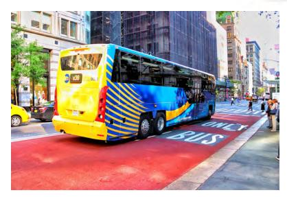
As part of the Fast Forward plan we are evaluating new bus designs. This new MCI Bus, with a first-of-its-kind, low-entry vestibule and an automated ramp, is currently being tested in service for the next 3 months. We look forward to gathering feedback from our customers.
